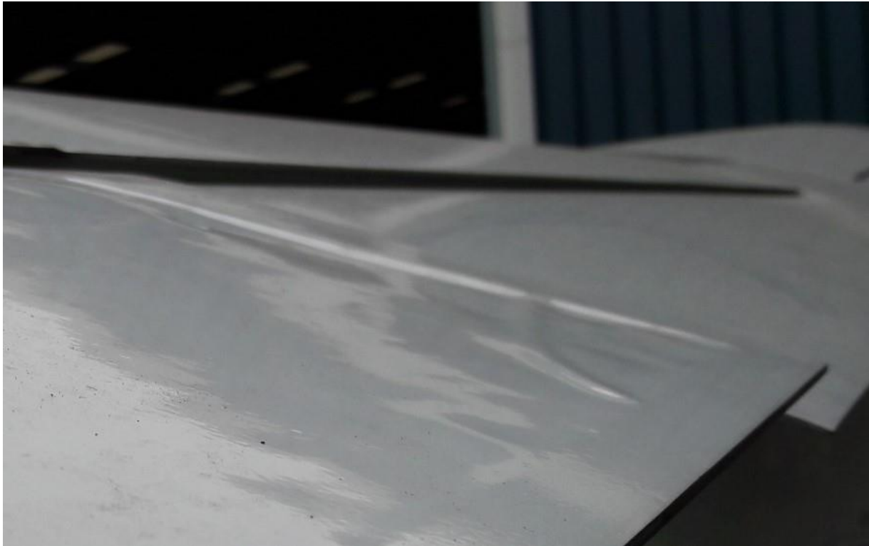
Shrinkage on the root of an aileron
