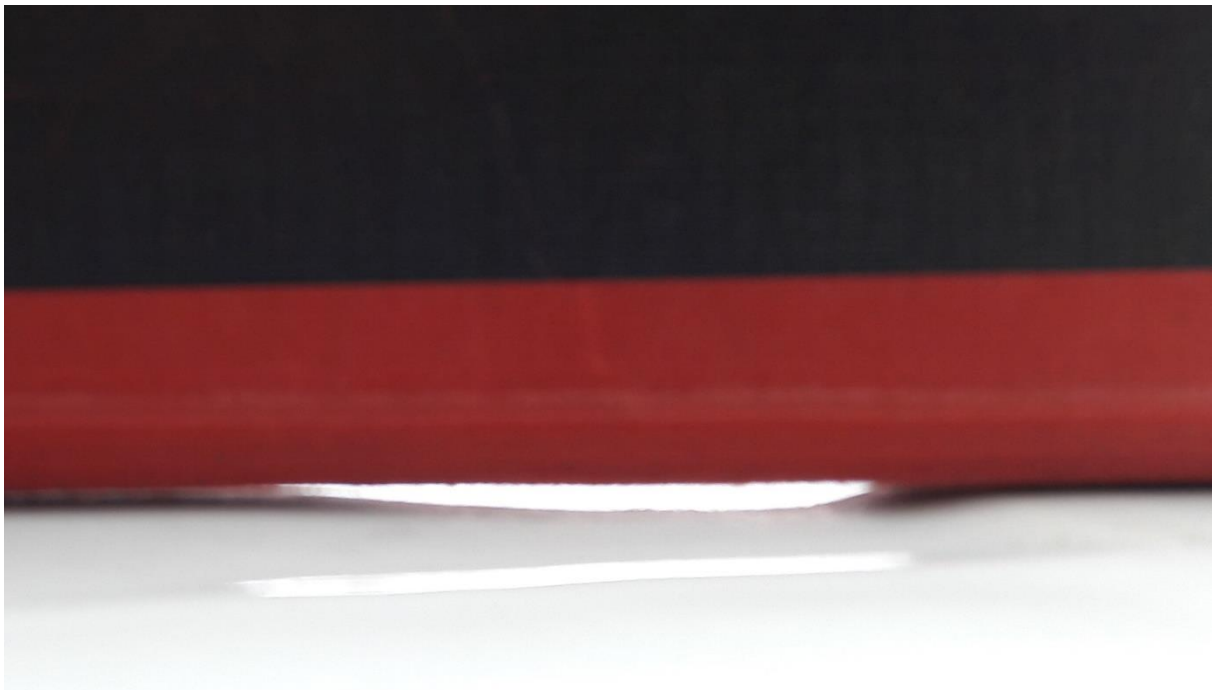
Shrinkage on the root of an aileron
