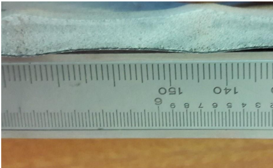
Severely damaged scrapped 8mm thick CT2K floor panel, 1mm deep shrinkage each side in 30mm. Was outside in the open for several years.
